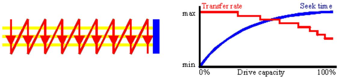
Traditional harddisks orders their capacity in ‘vertical’ mapping. The data is read/written from one cylinder first, starting at the top track down to the bottom, before the heads are moved to the next cylinder.
