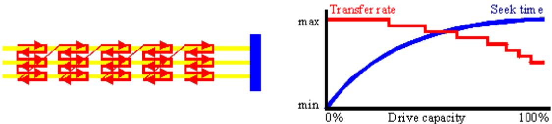
Some harddisks use a combination of ‘vertical’ and ‘horizontal’ mapping.
