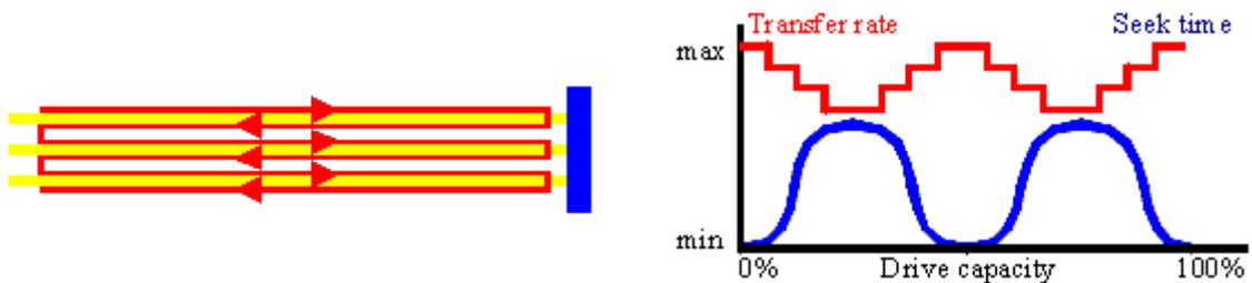
The ‘horizontal’ mapping. The data is read/written starting from the outer cylinder to the inner cylinder, before switching the heads to the next track.
