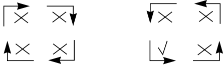
Figure 6: The corner-turns used by the restrictive route Y then route X router
