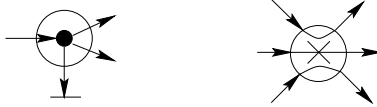
Figure 1: An active node (left) with an in-degree of 1 and an out-degree of 2 as well as a passive node (right) with an in- and out-degree of 3.
