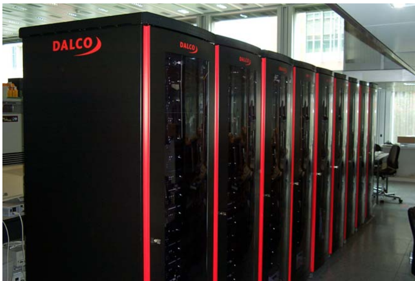
Figure 1: Front view of the Xibalba PC Cluster, the 128 nodes are mounted in 9 cabinets.
